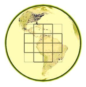
Figure 1: FOG field of view from ARSAT-1 position. The background Earth is a negative image of the city lights as obtained by NASA in visible light. The  $4 \times 4$  pixels are drawn on the Earth surface. The 4 corner pixels will be blinded.
